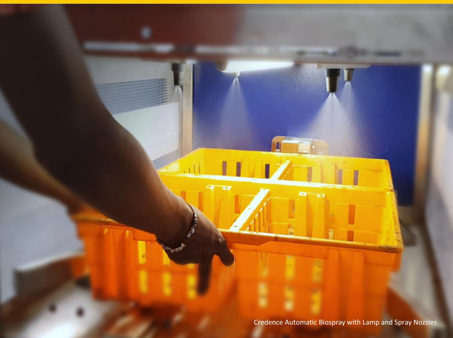
Credence Automatic Biospray with Lamp and Spray Nozzles
